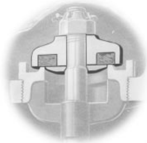
COMPOSITION DISC ASSEMBLY
